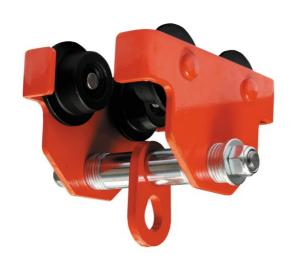
Anchor trolley ST 010 is designed as a portable anchor (attachment) point. It must be used with fall protection equipment. The trolley moves (drives) along a horizontal I-beam (rail). The rail must be fixed to a permanent structure. Anchor trolley ST 010 can be used with rails, 50 mm to 120 mm wide. The trolley provides protection for one person only.
