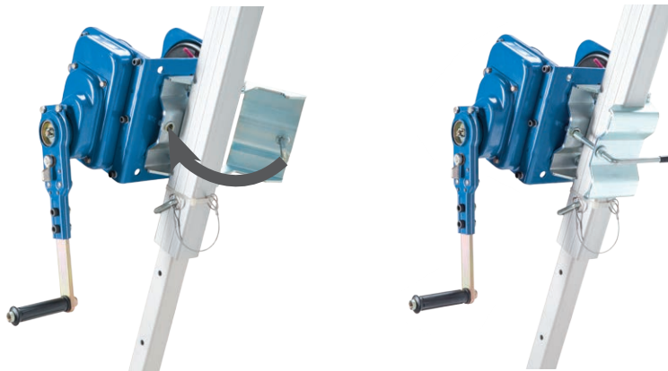
Mounting winch on tripod leg – clamp opened and closed.
