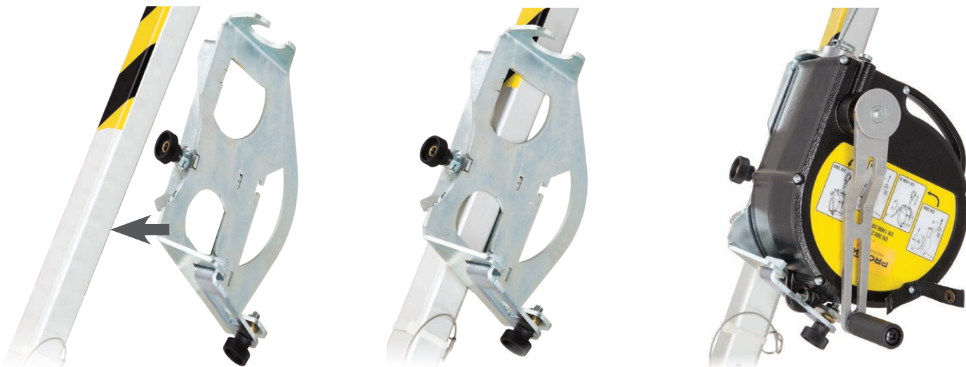
Clamp for mounting retractable type fall arrester CRW 200 on the tripod leg. According to the leg thickness, either clamp AT 173 or AT 174 is used. The clamp is simple to mount and is made of galvanized steel. Above is an example mounting of clamp AT 173 on tripod TM 9 leg.
