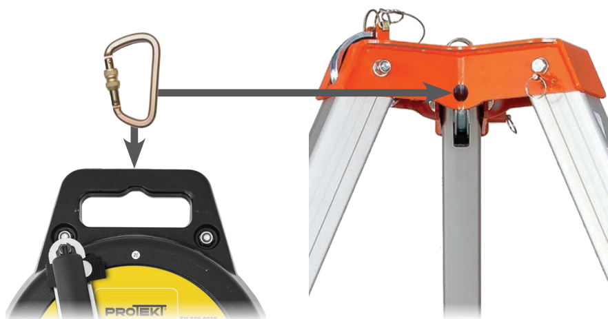
Side anchor point on tripod head can be used to attach fall arrester CRW 300 by means of connector AZ 017.
