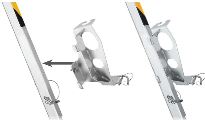
Clamp for mounting retractable type fall arrester CRW 300 on the tripod leg. According to the leg thickness, either clamp AT 171 or AT 172 is used. The clamp is simple to mount and is made of galvanized steel. Above is an example mounting of clamp AT 171 on tripod TM 9 leg.
